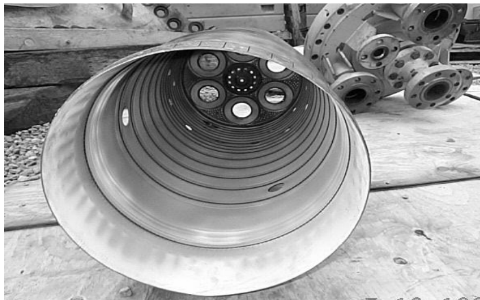
Figure 4 – A Combustion Chamber Can
